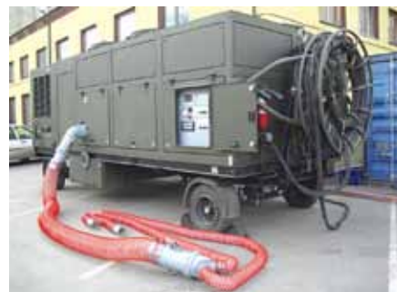
Ground air-condition unit AKA-1,0-30-1-1
